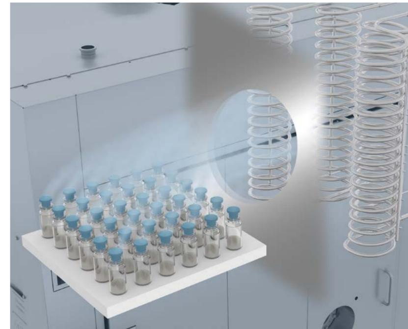
← Freeze-drying systems consist of components that are precisely matched to one another. Liquid quantities, valve size, cold surfaces and other factors are decisive. Laboratory and production systems should have conditions that are as identical as possible.
