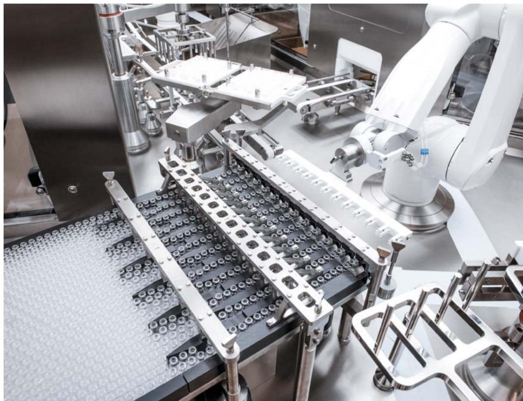
The system has two freeze-dryers: The isolators of the loading and unloading units are designed to process highly active substances. ↓
