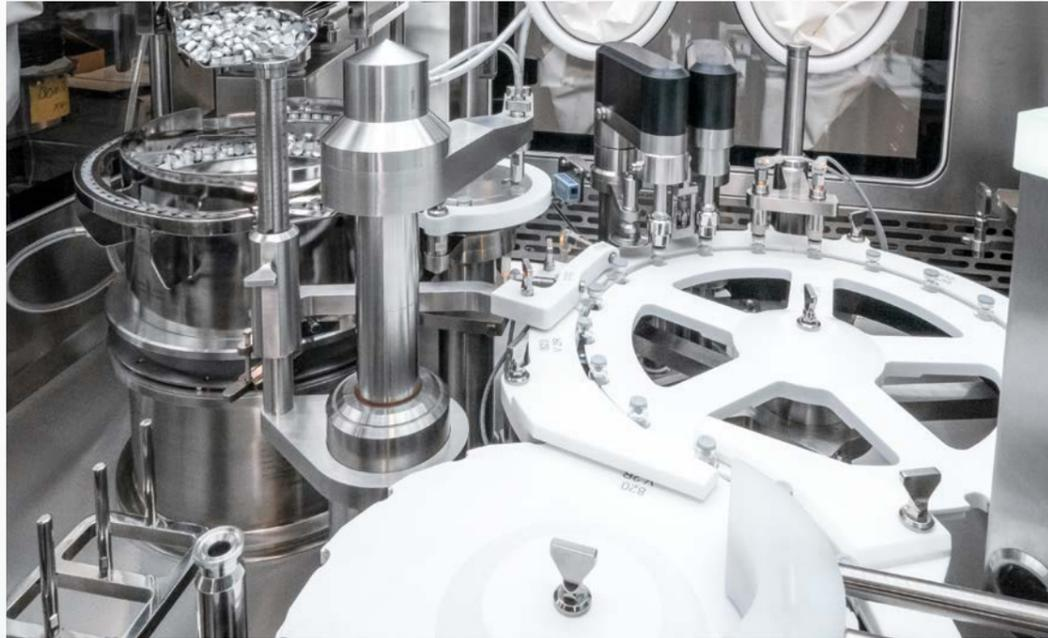
← Before the crimping process, a camera checks the exact position of the stoppers.
