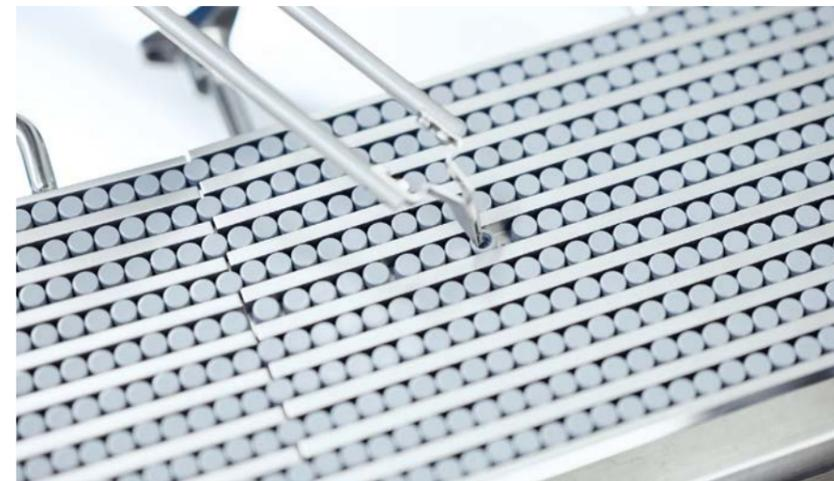
← Strategically, isolator systems with fewer glove ports make sense for medium and high-performance outputs. Shown: AI-controlled robotic solutions for inline troubleshooting of an incorrectly placed stopper.
